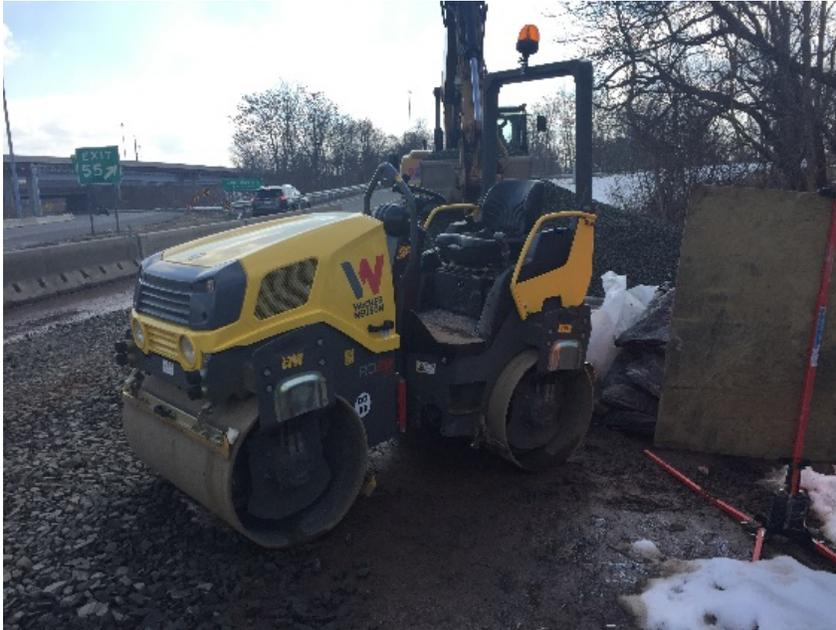
Low Profile Rollers and Mechanical Plate Tampers: Low Clearance for Bridge Reconstruction Projects, The lightweight doesn't displace the CMU facing blocks while compacting the backfill lifts.
