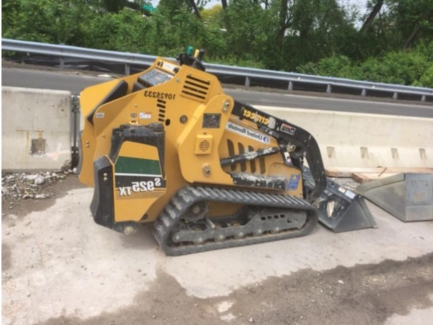
Walk Behind Rubber Tracked Loaders: With even lower profiles provide even more clearance than the skid steers and gain more access under existing bridges for reconstruction projects. Rubber Tracks allow for load distribution on and movement on loose graded No. 8 & 67 aggregate.
