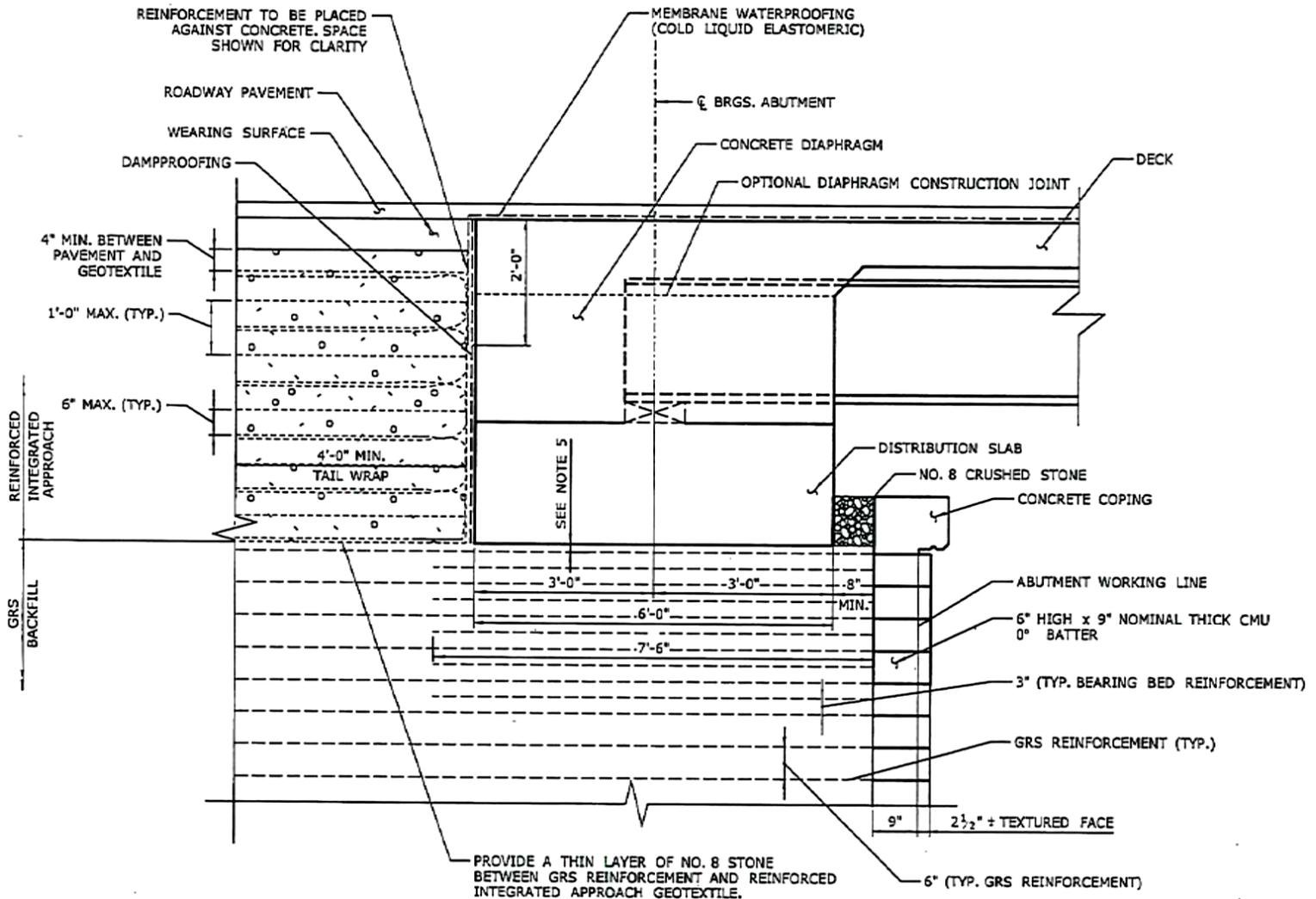
Bearing Bed Reinforcing Detail
