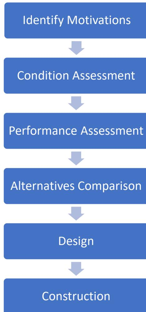
Figure 11: Steps in the Clarifier Rehabilitation Process
