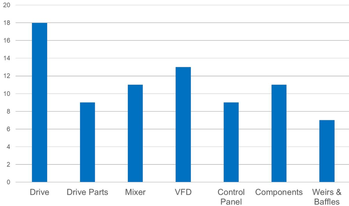
Figure 39: Typical lead time in weeks for clarifier items.
