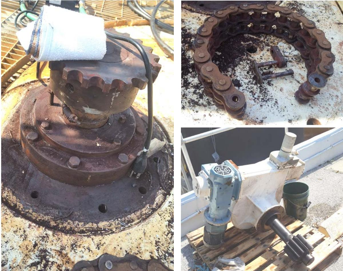
Figure 37: Disassembled drive unit for cleaning and inspection.
