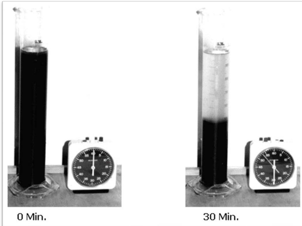
$$\text{SVI (mL/g)} = \frac{\text{Settled Sludge Volume (mL/L)}}{\text{Mixed Liquor Suspended Solids (g/L)}} \times 1,000$$
