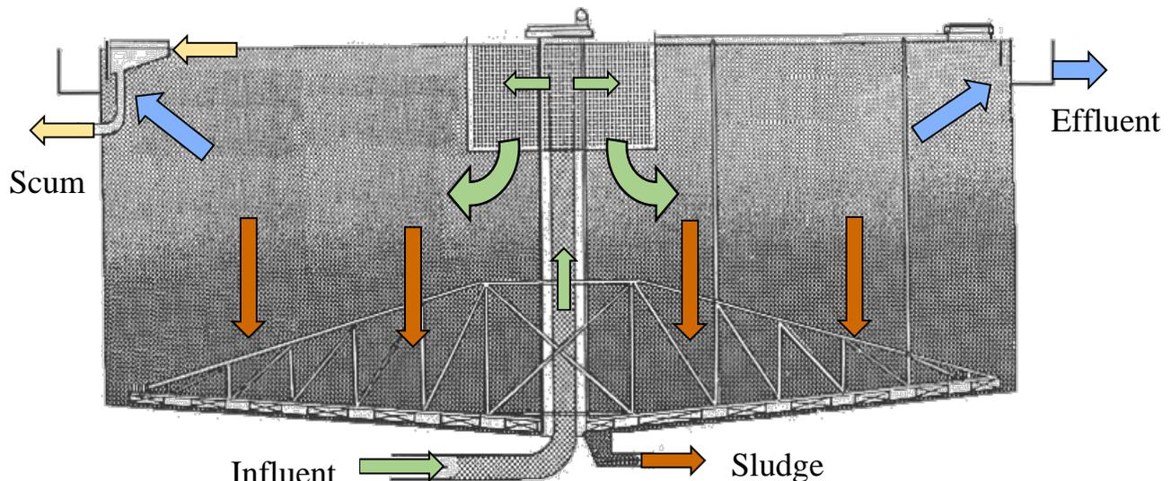
Figure 1: Flows in and out of a typical circular clarifier.
