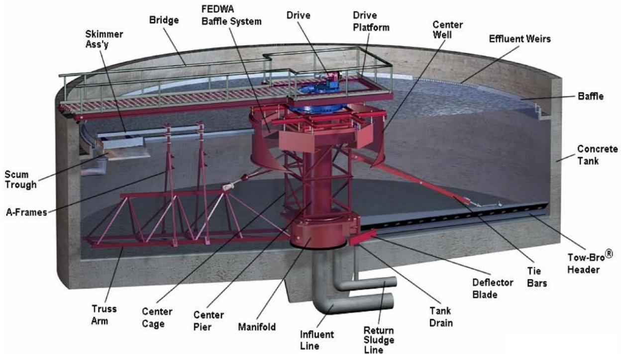
Figure 2: Typical components of a circular clarifier.
