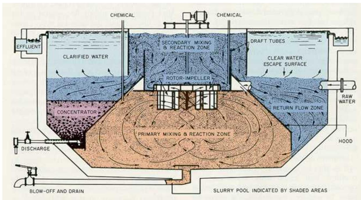
Figure 9: Zones in a typical solids contact clarifier.
