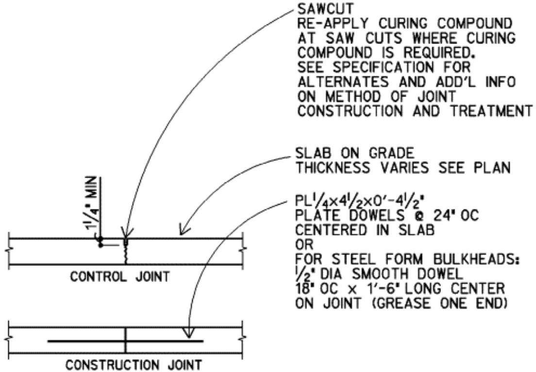
Fig. 29 - Typical details for control and construction joints in a concrete slab
