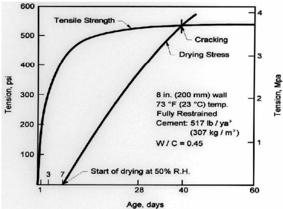
Fig. 25 - Relationship between tensile strength and drying stress over time (United States Nuclear Regulatory Commission)
