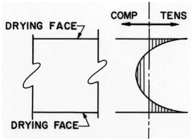
Fig. 19 - Stresses in a slab with a top and bottom drying face – (United States Nuclear Regulatory Commission)
