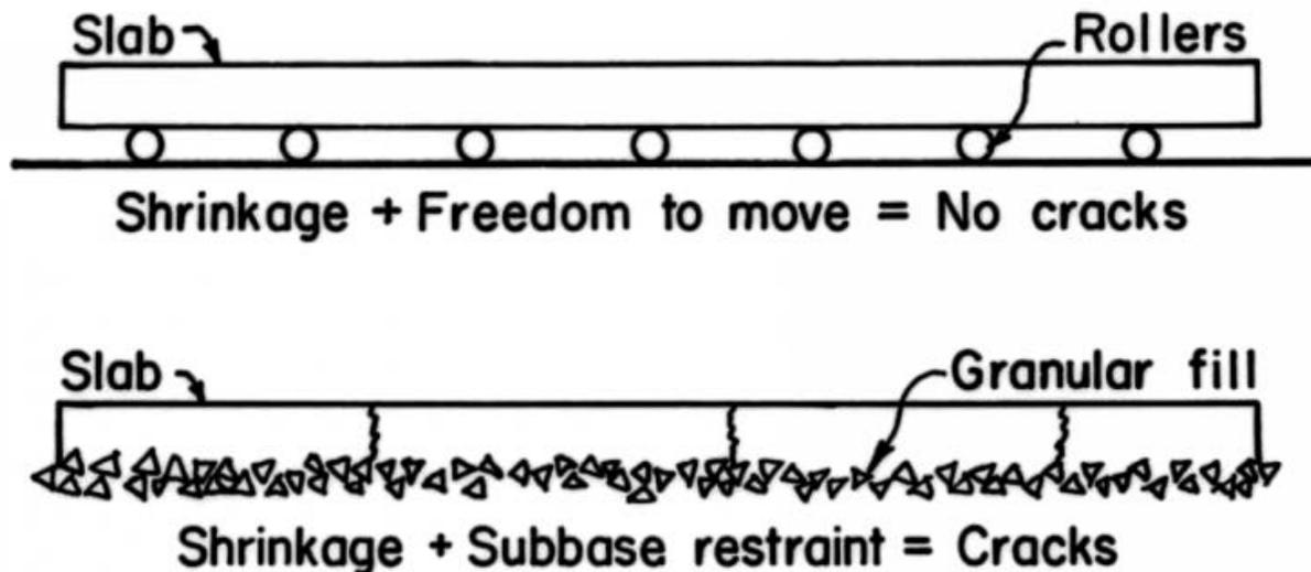
Fig. 20 - Cracking due to restraint of a shrinking slab (United States Nuclear Regulatory Commission)
