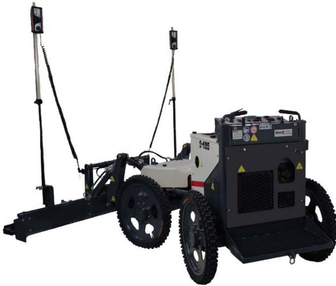
Fig. 15 - Lightweight ride-on laser screed (<https://www.somero.com/products/ride-on-screeds/s-485-laser-screed-model/>)
