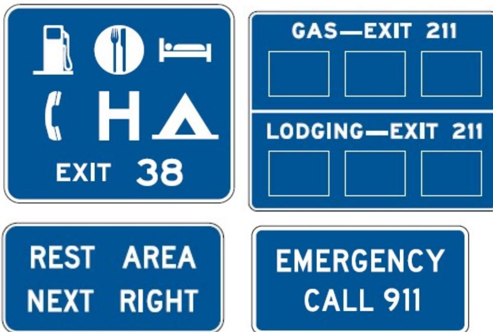
Figure 31. Example of general service and specific service signs for a freeway
