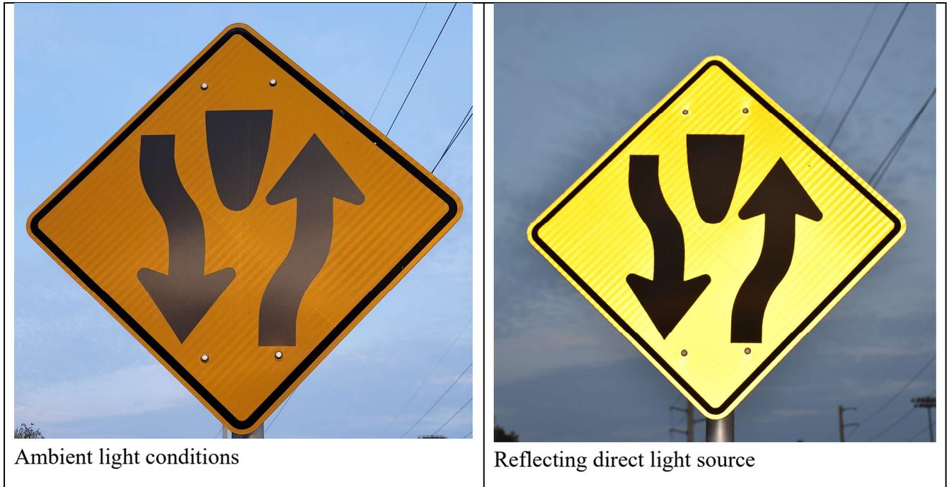
Figure 4. Example of retroreflection sign material
