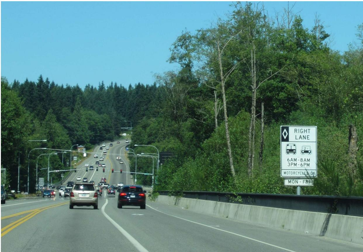
Figure 28. High occupancy vehicle lane sign example
