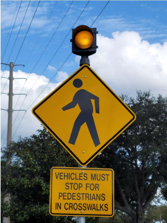
Figure 11. Supplemental flashing beacon
