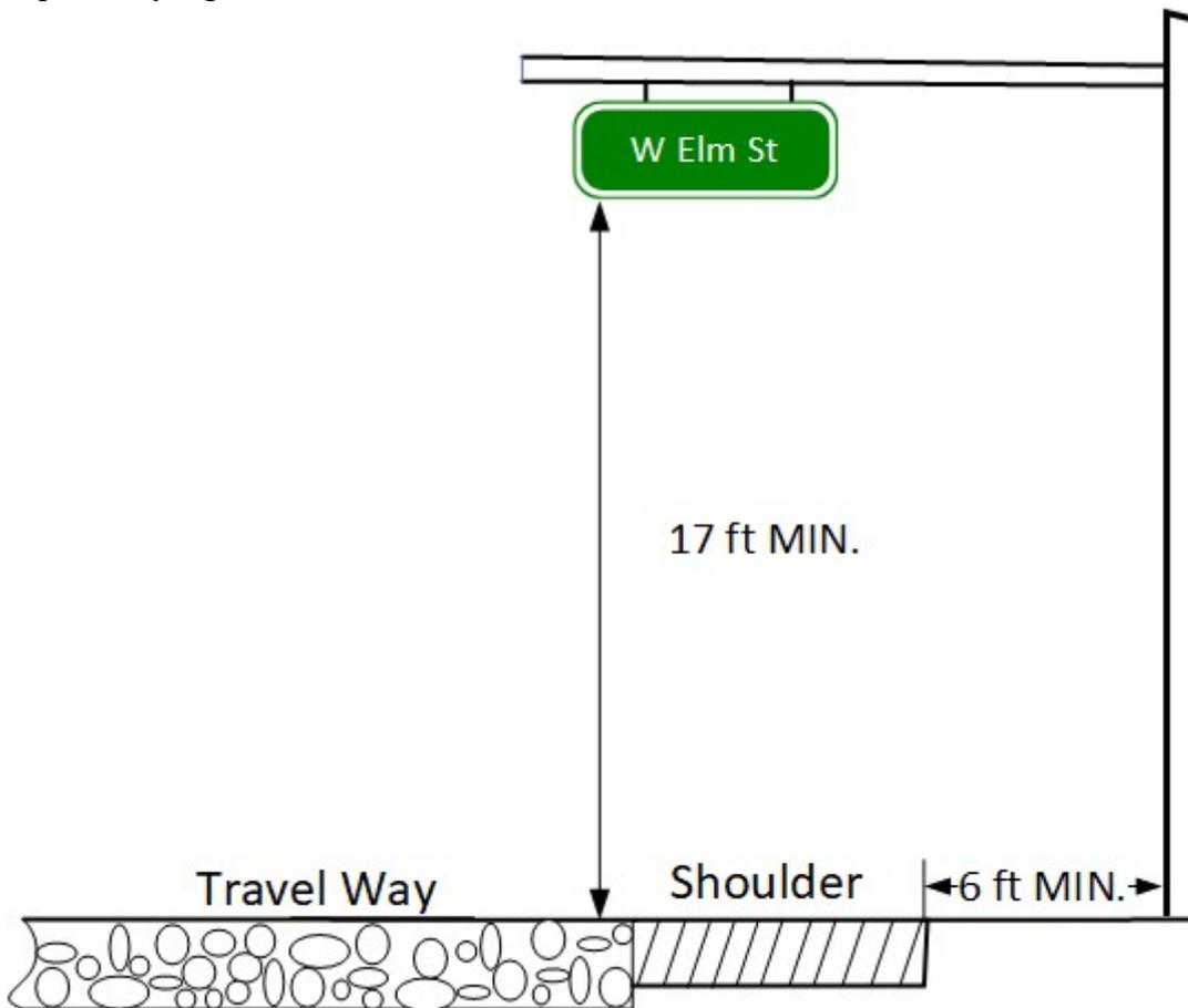
Figure 17. Overhead sign support lateral placement
