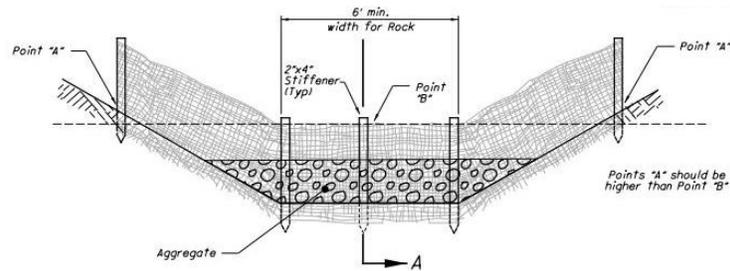
**CROSS-SECTIONAL VIEW OF FLAT BOTTOM DITCH**
