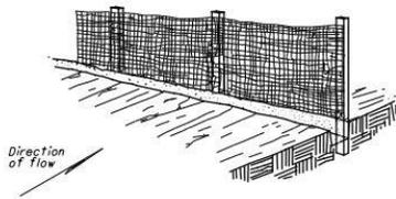
**Silt Fence Installation**
