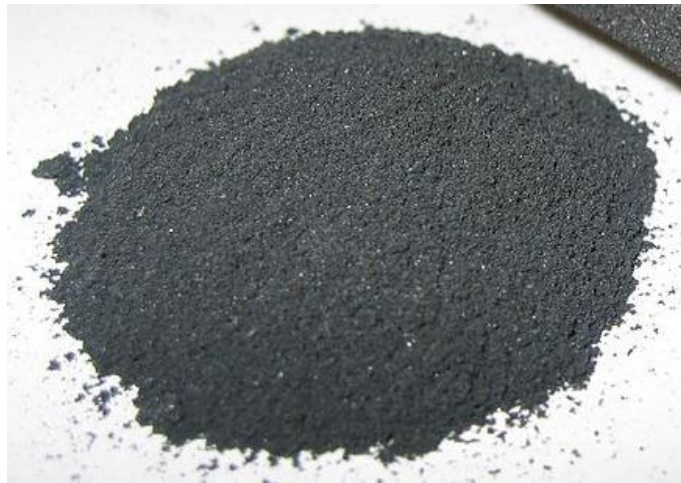
Figure 12: Example of powdered activated carbon media.
