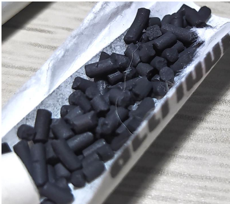
Figure 14: Example of extruded activated carbon media.
