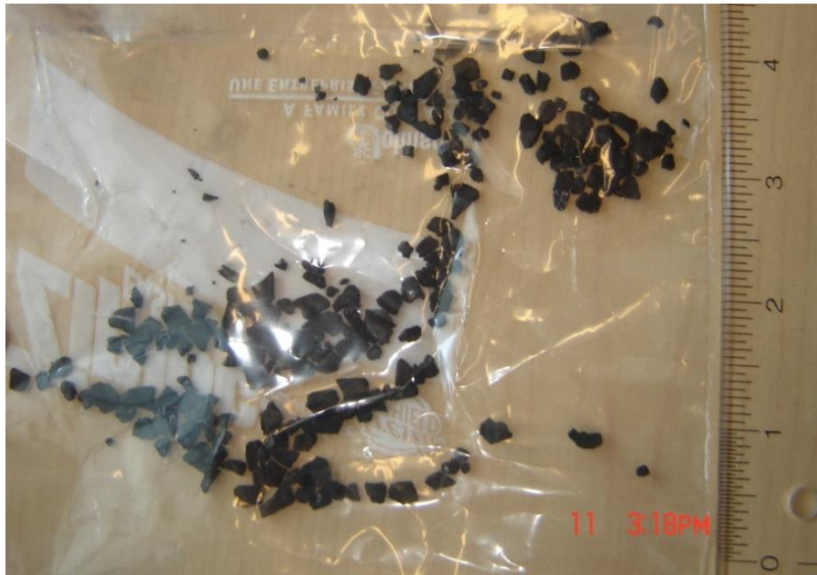
Figure 13: Example of granular activated carbon media.
