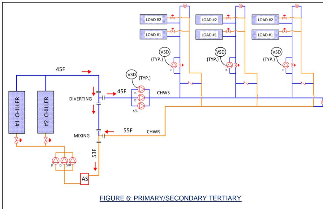
Variable Speed Drives may be applied to these systems (shown above) in which case each Secondary Pump operates based off of loop differential pressure. As with the previous example, the Primary Pumps typically operate at constant speed with these systems. The chillers stage on/off as described with the classic model.
