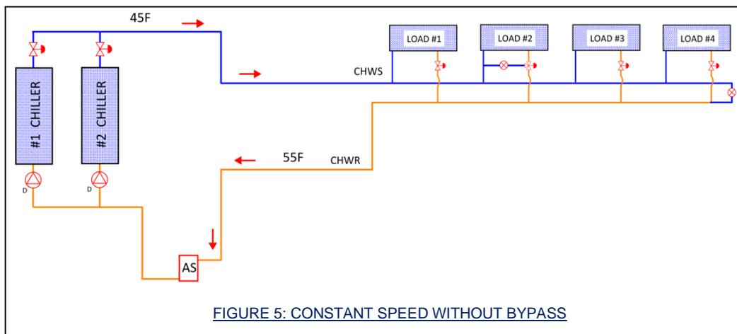
The control logic is the same as the classic Primary/Secondary piping model and we have an opportunity to isolate flow through the #1 Chiller or #2 chiller when they sense a reduced differential pressure due to reduced flow rate or when commanded off by the Chiller Control Panel. In either case, there is a light load condition so there is an opportunity to increase flow rate in the lead chiller which will benefit its operation.
