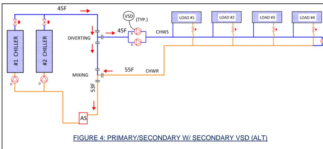
The control scheme associated with these piping arrangements can become more complex and include more monitoring controls (e.g., the decoupler must be monitored for proper flow direction). If the first “T” fitting becomes mixing, then the loop will see water temperatures
