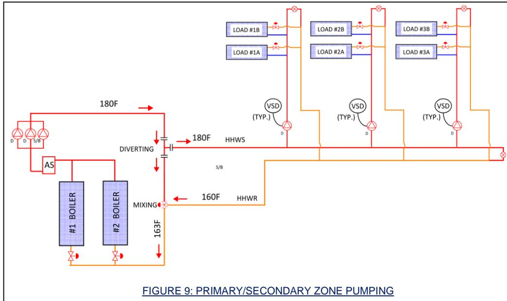
Control of the primary equipment is the same as described previously. Secondary Loop zone pump control is based on differential pressure for variable pumping systems. These systems must be “tuned” since each zone pump temporarily draws from other zones until which time the Primary Loop pump(s) can achieve pressure.
