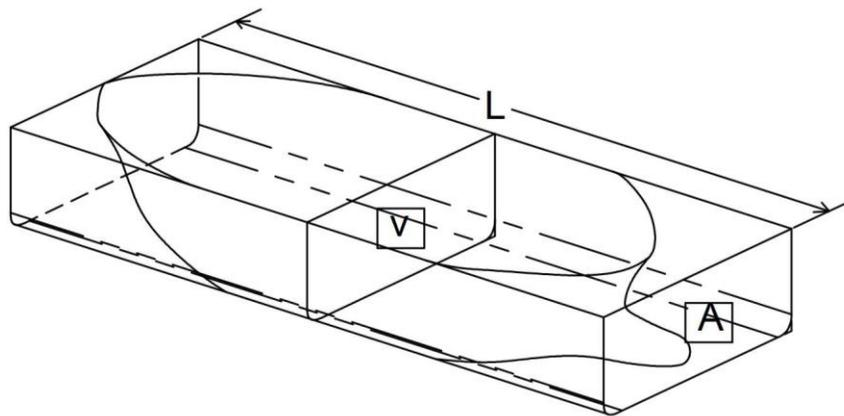
Figure 5: Prismatic Coefficient
