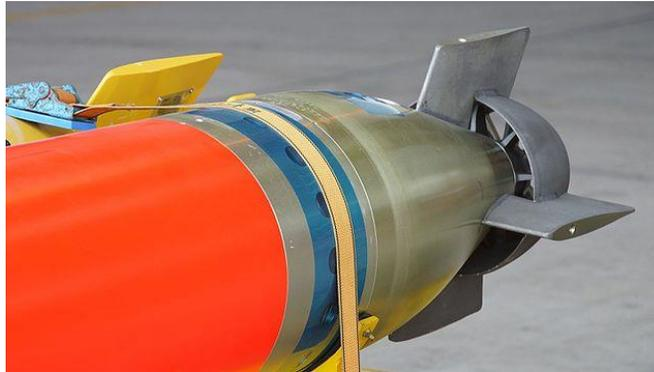
Figure 17: Pumpjet on a torpedo
