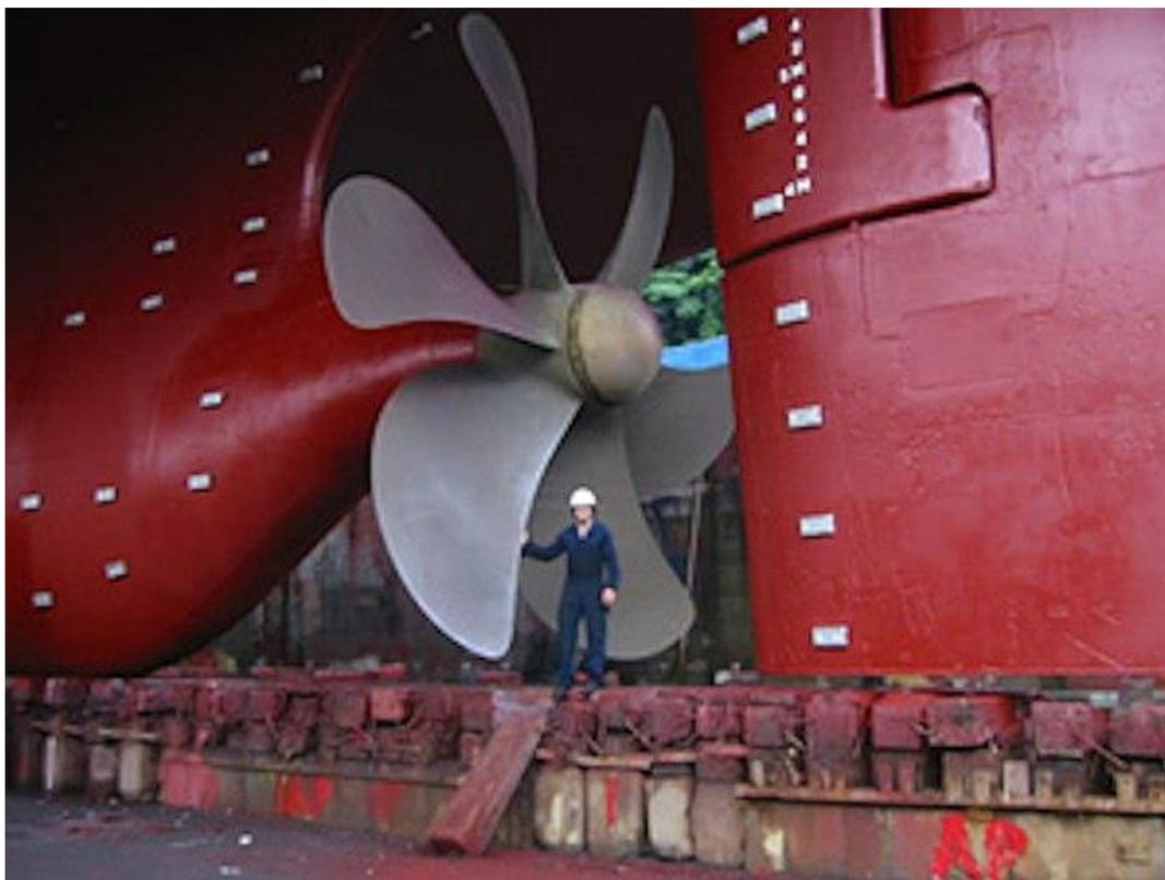
Figure 12: Conventional Ship Propeller
