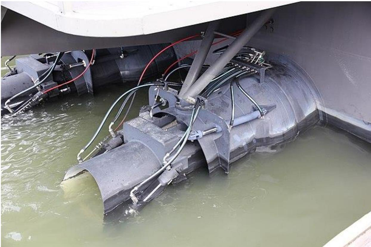
Figure 16: Waterjet with steerable nozzle but no bucket
