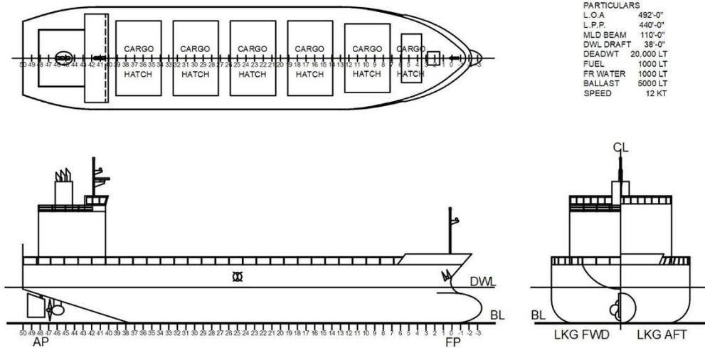
Figure 3: Azipod Drive Bulk Carrier
