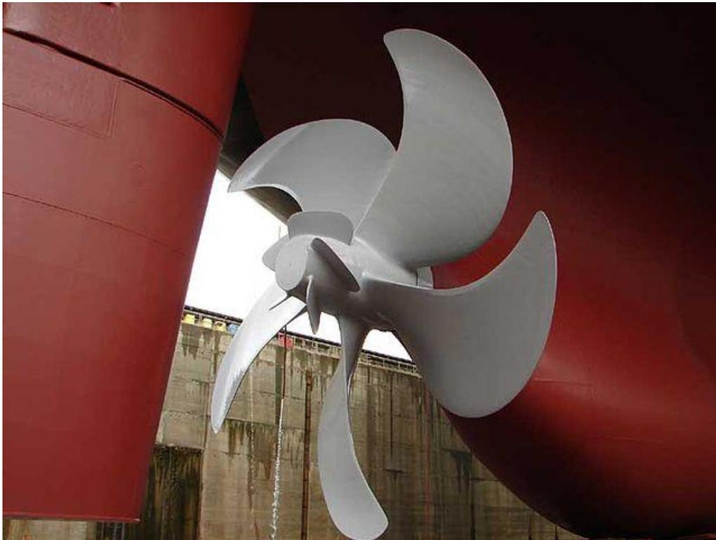
Figure 13: Conventional Ship Propeller with Hub Vortex Reducer Cap
