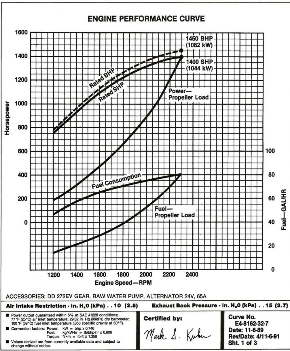
Figure 8: Typical Diesel Power vs RPM Graph For A High-Speed Vessel
