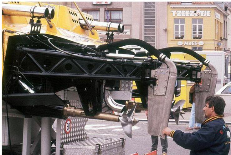
Figure 14: Surface-Piercing Propellers
