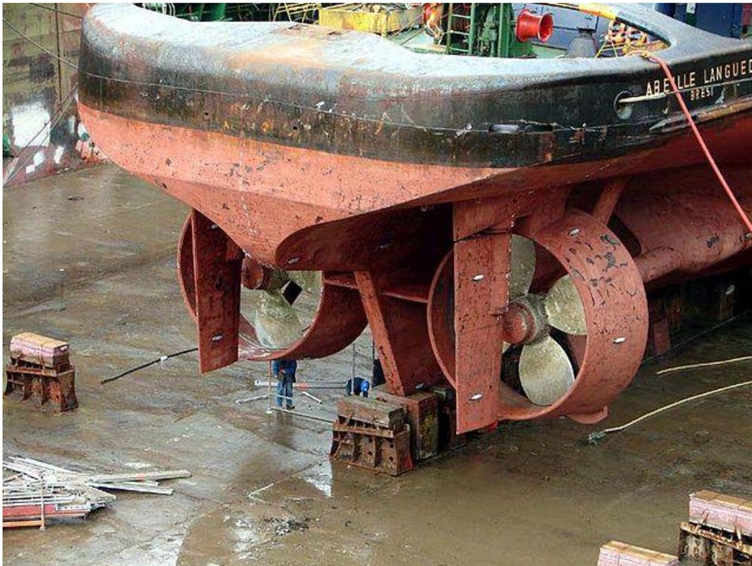
Figure 15: Nozzle Propellers on a Tug
