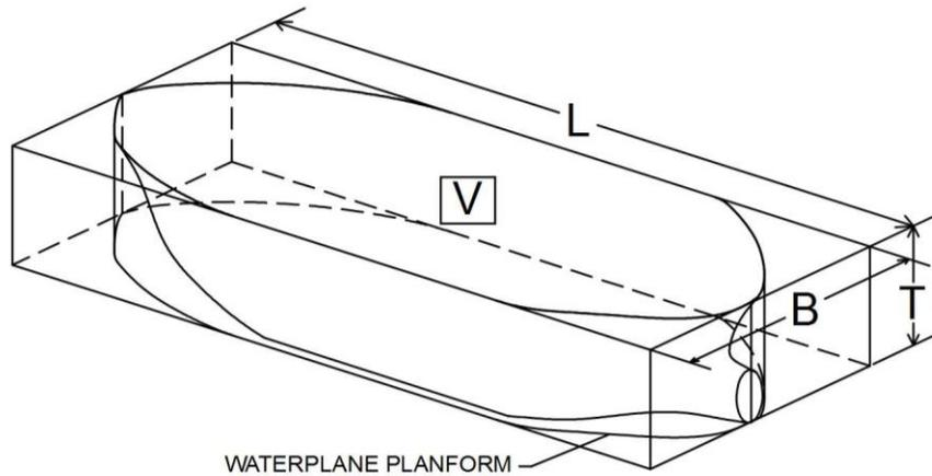
Figure 7: Vertical Prismatic Coefficient
