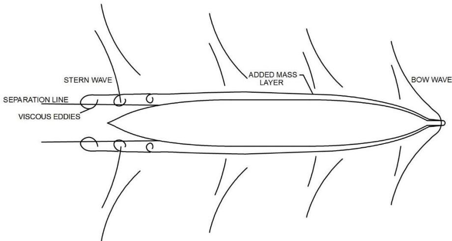
Figure 11: Wave pattern of ship with a bulbous bow
