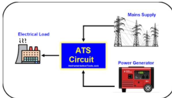
The single disadvantage to the ATS is that the generator will only generate power to support the load connected to the ATS. This eliminates the ability to effectively use “excess” generator capacity. However, many would not consider this a disadvantage at all since the primary and often only reason for the generator is to provide power for the Critical Facility when utility source is unavailable.
