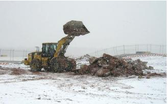
Loaders are one of the most versatile pieces of equipment at any Heavy Civil Construction Project and therefore they are found on almost every site. Some are tractor-loader-backhoes, although most are straightforward front-end loaders.
