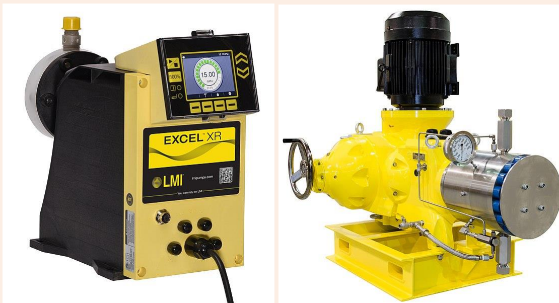
Figure 12: Examples of mechanically actuated diaphragm pumps. Left: Small metering pump with built-in speed control, control screen, and a standard outlet plug. Right: Large metering pump with a vertical motor designed for pressures up to 15,000 psi. The wheel is for manual stroke adjustment.
