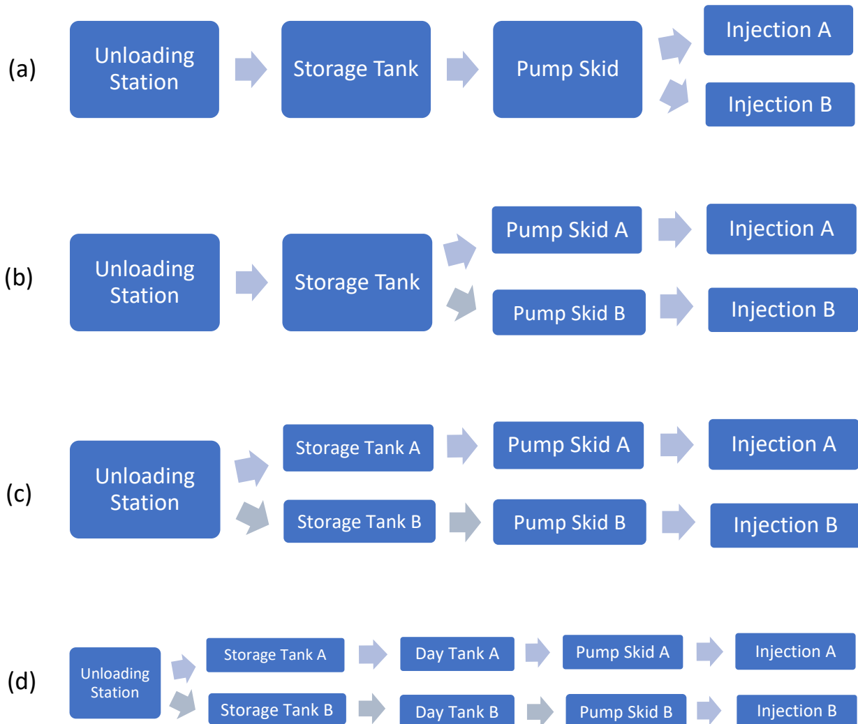
Figure 4: Four possible block flow arrangements for a chemical feed system with two injection points, in order from least redundancy (a) to most redundancy (d).
