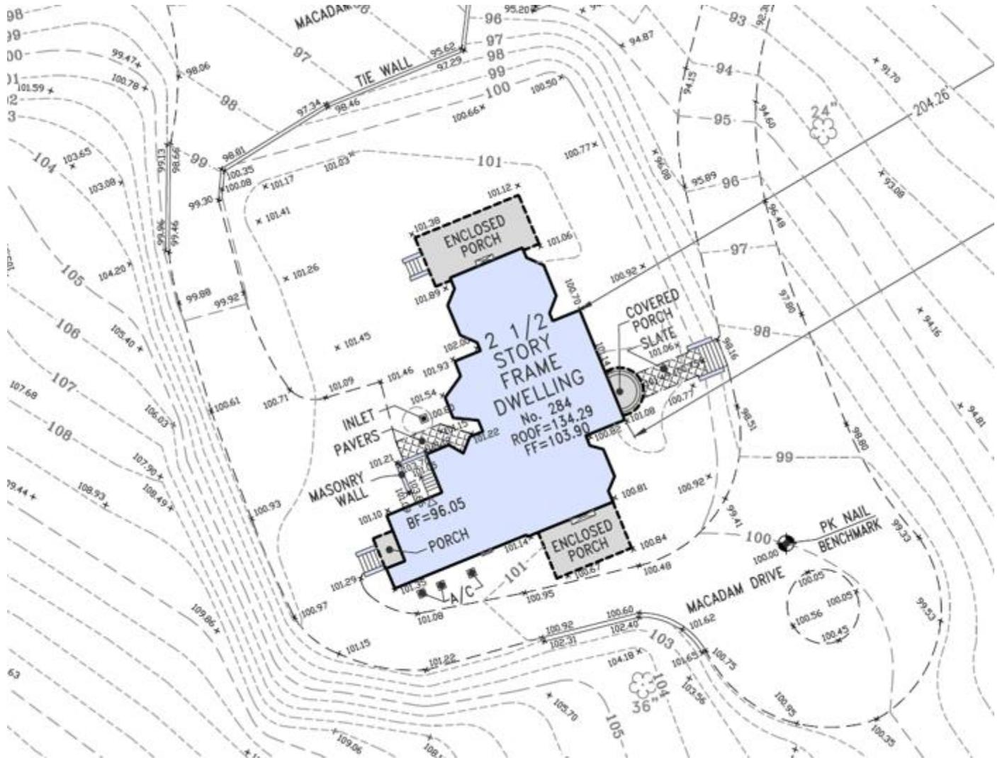
Note that often an assumed datum (rather than using sea level datum) is used for topographic mapping. This is the case in the topographic survey shown above. A datum of 100 was assumed at a point in the road in front of this dwelling. (This can be seen in the label “PK Nail Benchmark” in the screen shot above).
