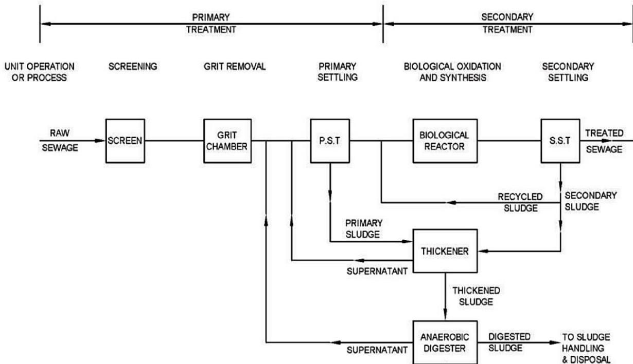
Figure 2: Wastewater treatment system with primary and secondary processes. P.S.T. is primary sedimentation tank and S.S.T. is secondary sedimentation tank.
