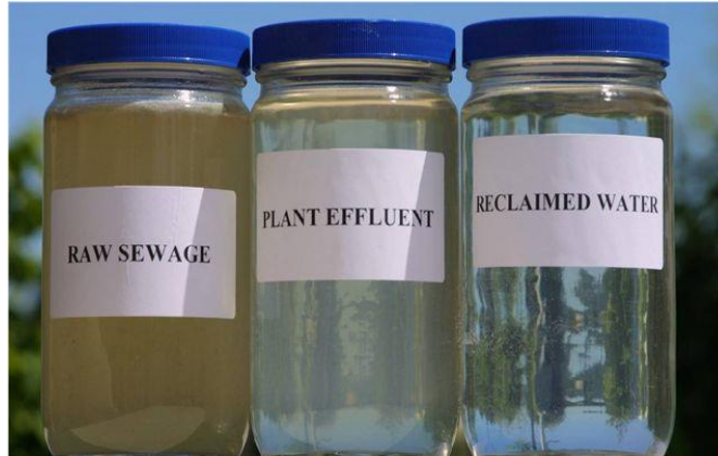
Figure 8: Visual comparison of the color and turbidity differences in raw municipal wastewater (left), treated effluent (center), and advance treated reclaim water (right).
