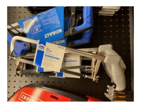
The main missuse of hacksaws is utilizing the wrong blade or not properly tightening the blade when in use. Most blades will cut through the intended material but certain blades perform better than others for certain jobs.
