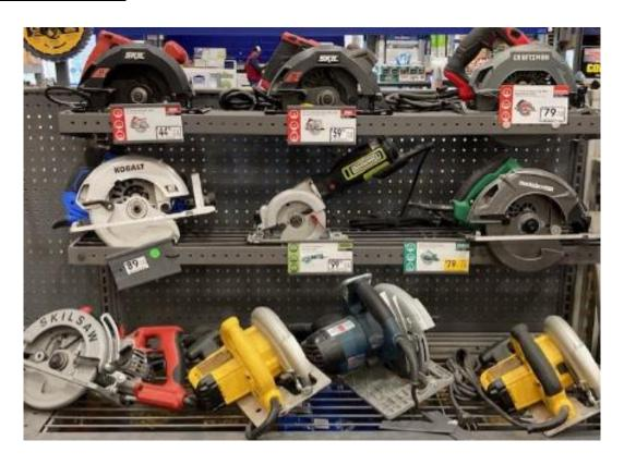
What hazards are most often associated with the use of power saws? Experience shows that most injuries from their use are eye injuries from saw dust and foreign objects, and cuts from contact with the blade. There is also the potential for electric shock from improper use or conditions.
