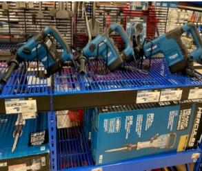
Jackhammers probably cause more serious injuries in heavy civil construction than any other hand tool. They cause serious back injuries, eye injuries, and the occasional foot injury. Extended exposures can lead to hearing loss, and the vibrations /impacts can lead to hand wrist and arm damage. They create silica dust from the demolition activities and precautions must be taken for these risks but they will be the subject of a separate course in Silica Exposure Construction Safety.
