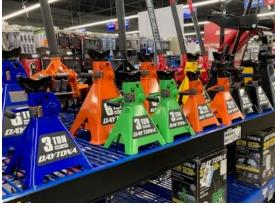
Jacks are a little more specialized than the previous tools but they must be used correctly or the consequences can be catastrophic. Jacks need to be on firm, level, and stable ground. Do not allow workers underneath a jack only supported load. The jack needs to have the load capacity clearly identified on the tool and should have a position stop to prevent overtravel of the lifting cam. Lubrication and maintenance must be scheduled and followed by the manufacturer's requirements.
