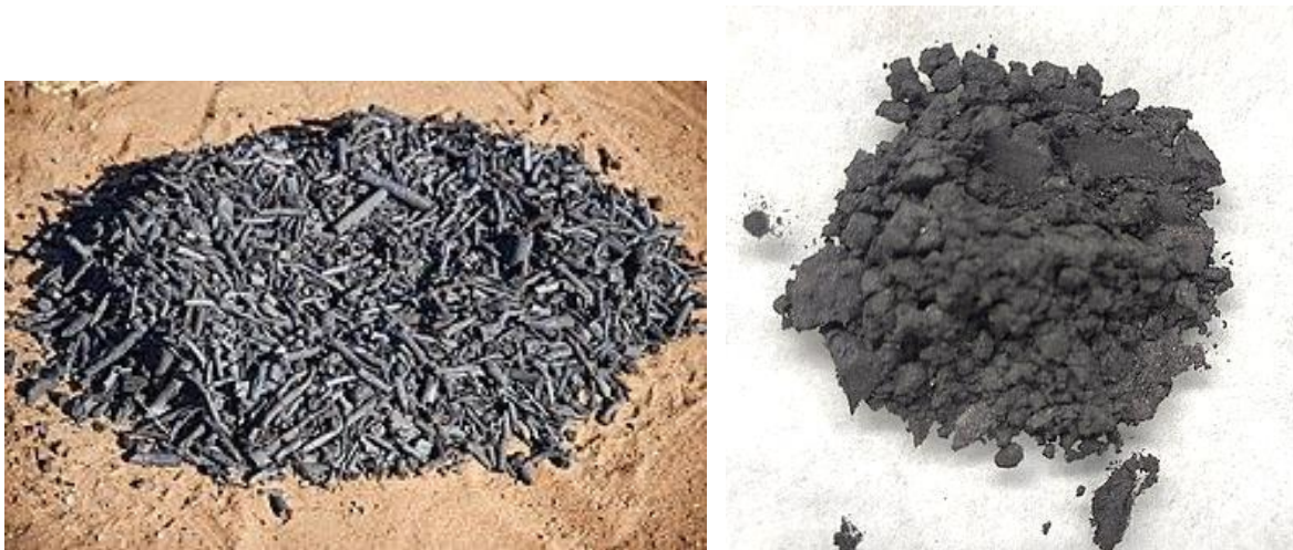
Figure 21: Biochar (left) and activated carbon (right) which can be mixed with biosolids.
