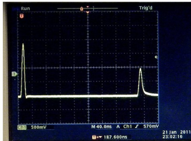
Figure 4: TDR with Open Termination
